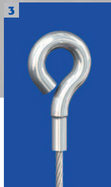
3 Wire eyelet Ø 6 mm WLL 10 kg
