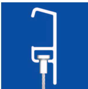
Coupling with T-sleeve 02, inserted laterally. See page 23
