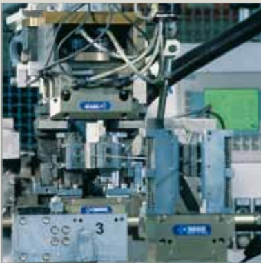
Fully automatic cable-production with testing
