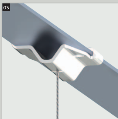
03 Track-Clip ›Quick‹ white for cables ø 1,0 - 1,5 mm with ball sleeve 35 WLL (DIN 18168) 25 kg Art. no. 029.006.356
