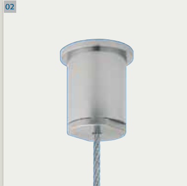
Ceiling attachment M13x1; M6i short and screw cap M13x1 with bore 2.4 mm SW 14
